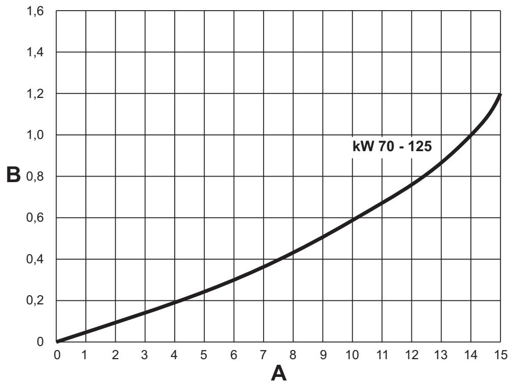
fig. 90 - Pressure loss diagram models 70 - 125
