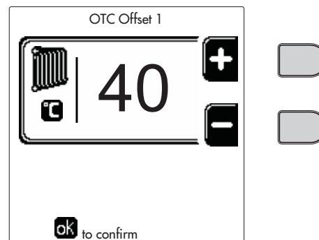
fig. 29- Parallel curve offset
