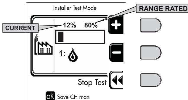
fig. 64 - Test mode (example heating power = 80%)
