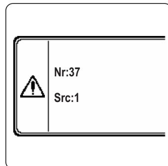
fig. 32- Module 1 insufficient system pressure fault
