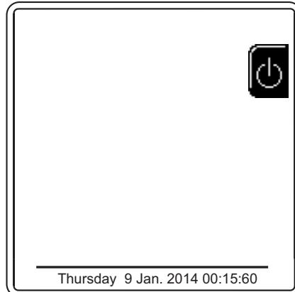
fig. 11- Turning the boiler off
