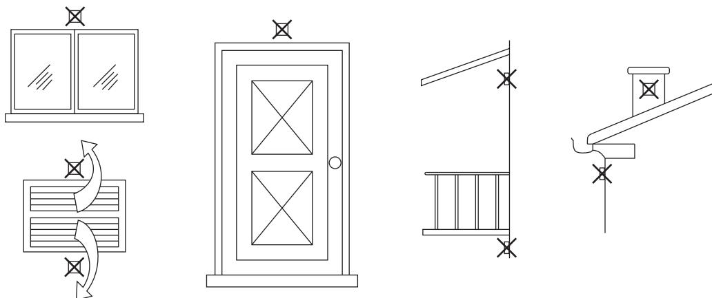
**fig. 54- Positioning of external probe not recommended**
