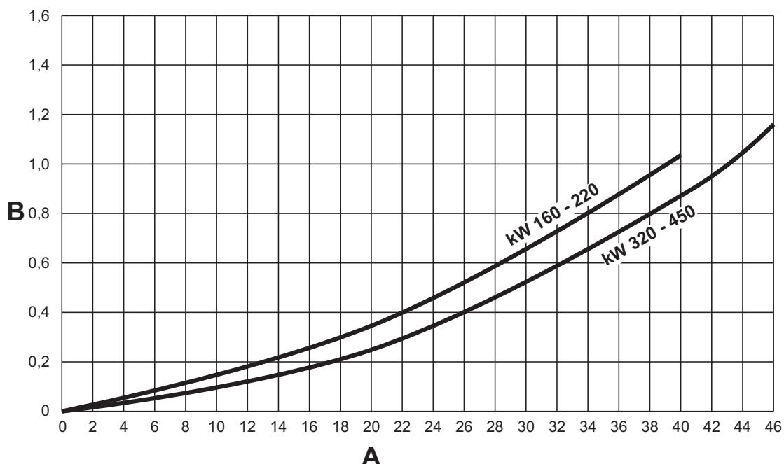
fig. 91 - Pressure loss diagram models 220, 320 and 450
