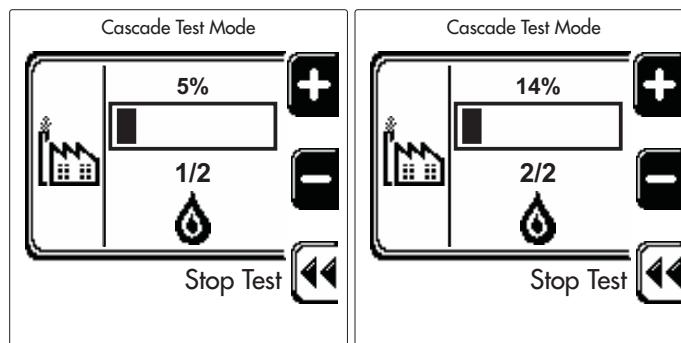
fig. 66 - Cascade TEST mode (example with two modules)
